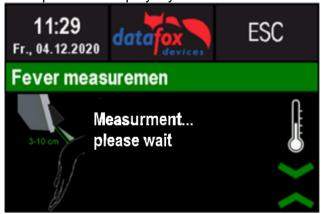
In the display designer, the images are to be specified as follows if the option is selected. Firstly, the image for the explanation (in the left-hand area) and for the thermometer (in the right-hand area).
