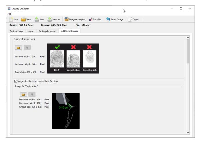
If the option "Images for the field function for fever control" is not selected, the images will not be transferred to the unit, even if a corresponding fever control function has been installed in the unit. If the option is selected, the images are only transferred to devices with a built-in fever control function.
