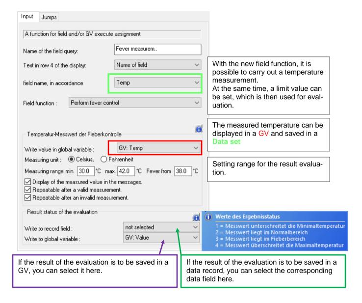
The measured temperature is stored in the record description field "Temperature" after successful completion of the function in this example.
