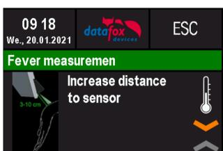
In this case the wrist is too close to the sensor. sensor away.
